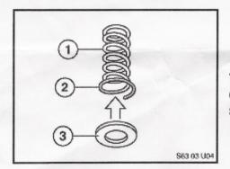
Temporarily hold the washer (3) in place on the spring (1) using dum-dum (or equivalent) applied to the area shown (2).
