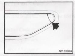
Excess spring tension caused by the 82N retaining springs may cause stress cracks in the third brake lamp.
