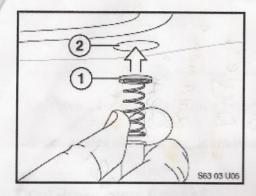
washer (1) to the lamp mounting stud through the trunk panel hole (2) as shown.
